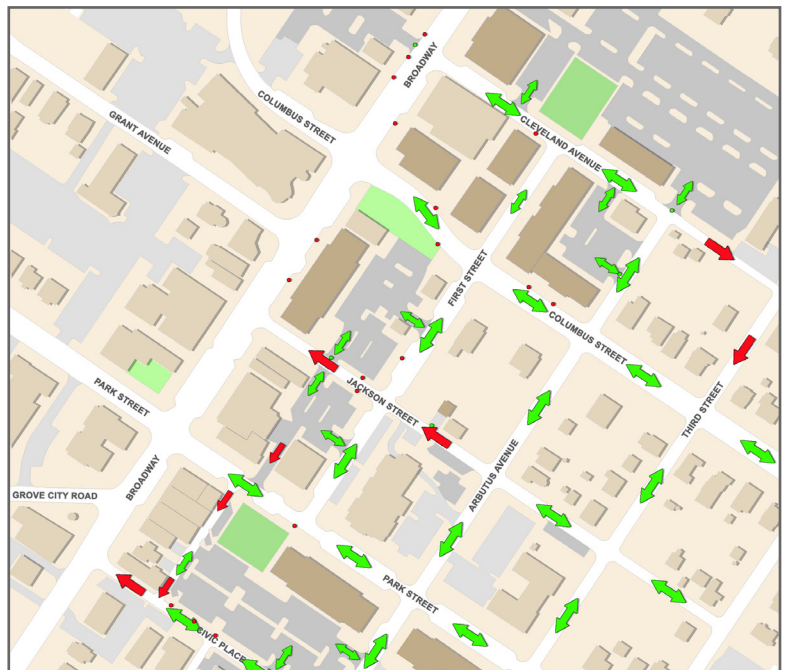
Proposed Directional Traffic Flow and Vehicular Access Modifications East of Broadway
