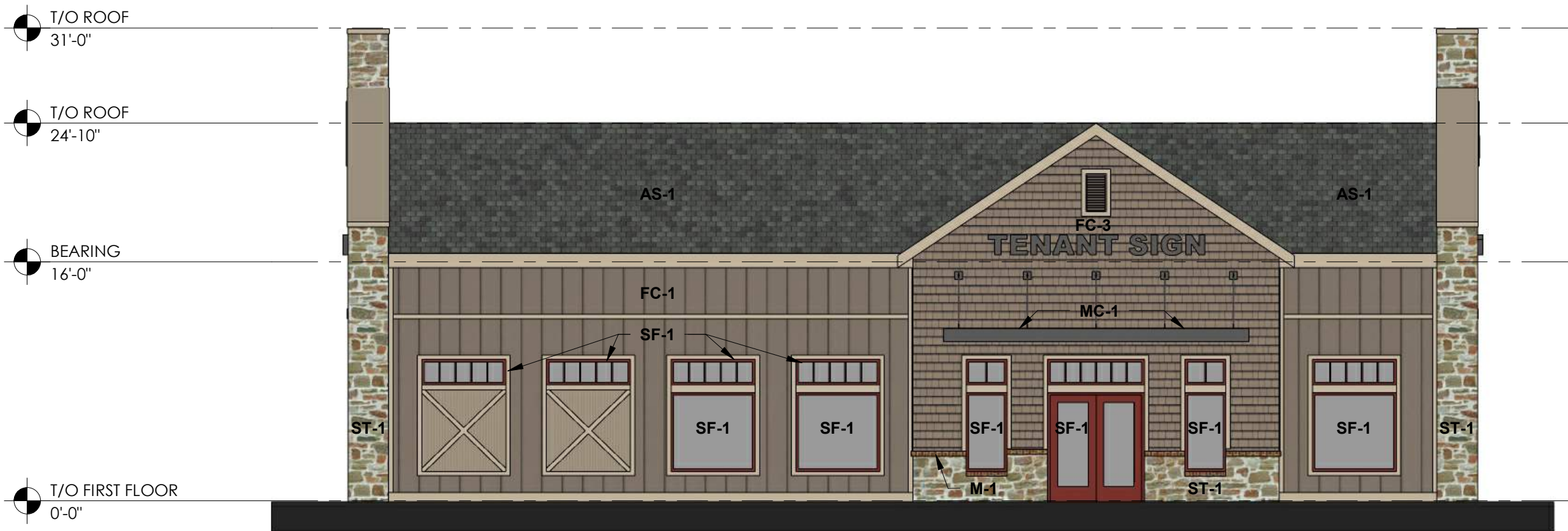
2 BUILDING C NORTH ELEVATION 1/8" = 1'-0"
