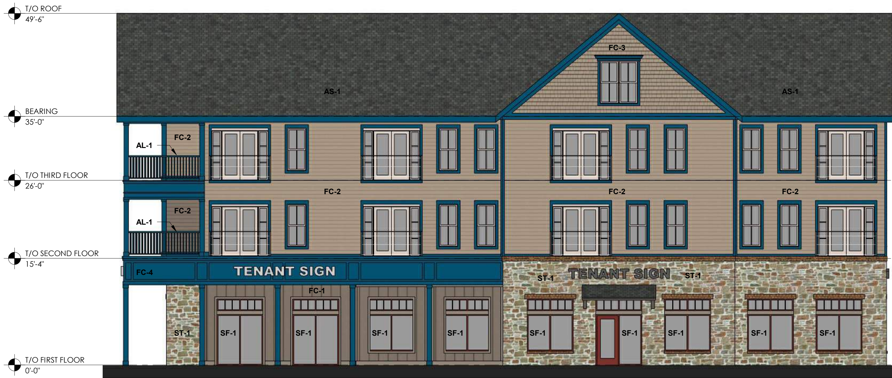
2 BUILDING A NORTH ELEVATION 1/8" = 1'-0"
