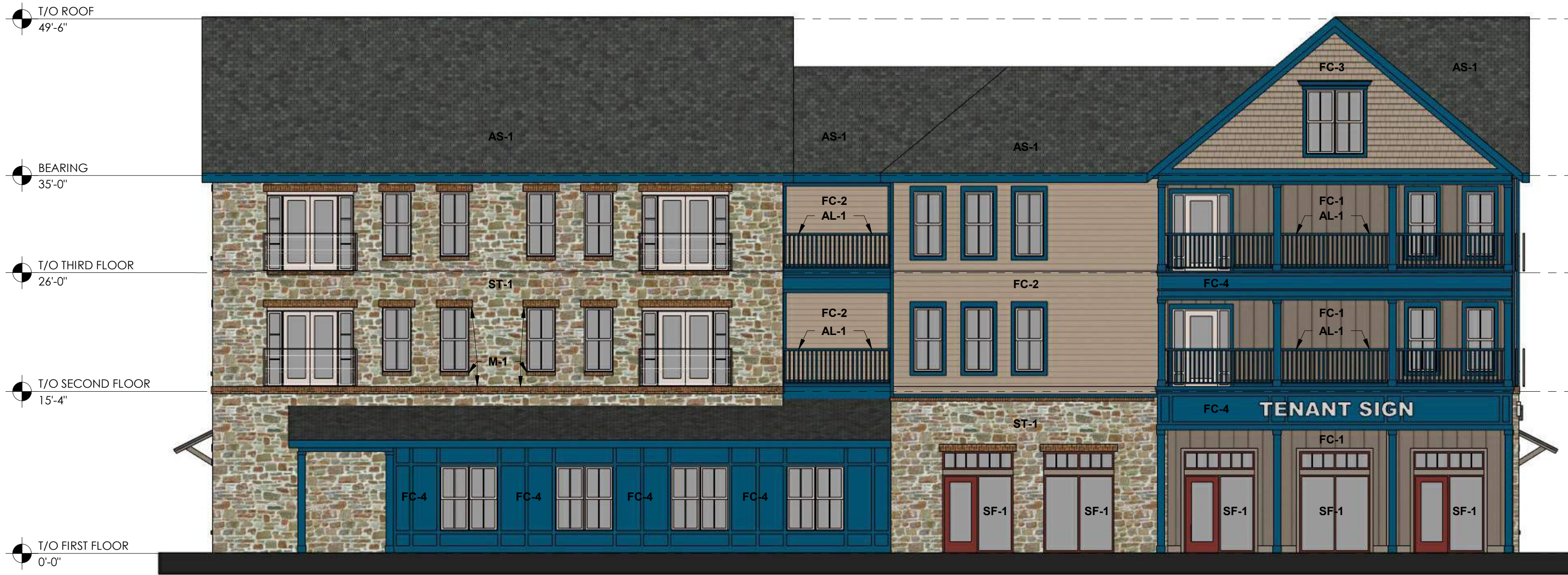
3 BUILDING A EAST ELEVATION 1/8" = 1'-0"
