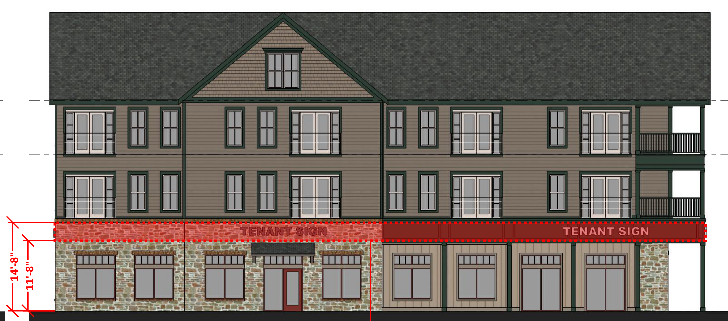
① BUILDING B SOUTH ELEVATION 1/8" = 1'-0"
