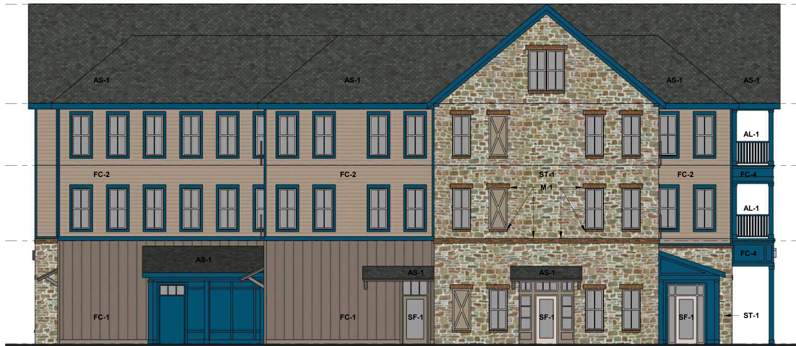
1 BUILDING A SOUTH ELEVATION 1/8" = 1'-0"
