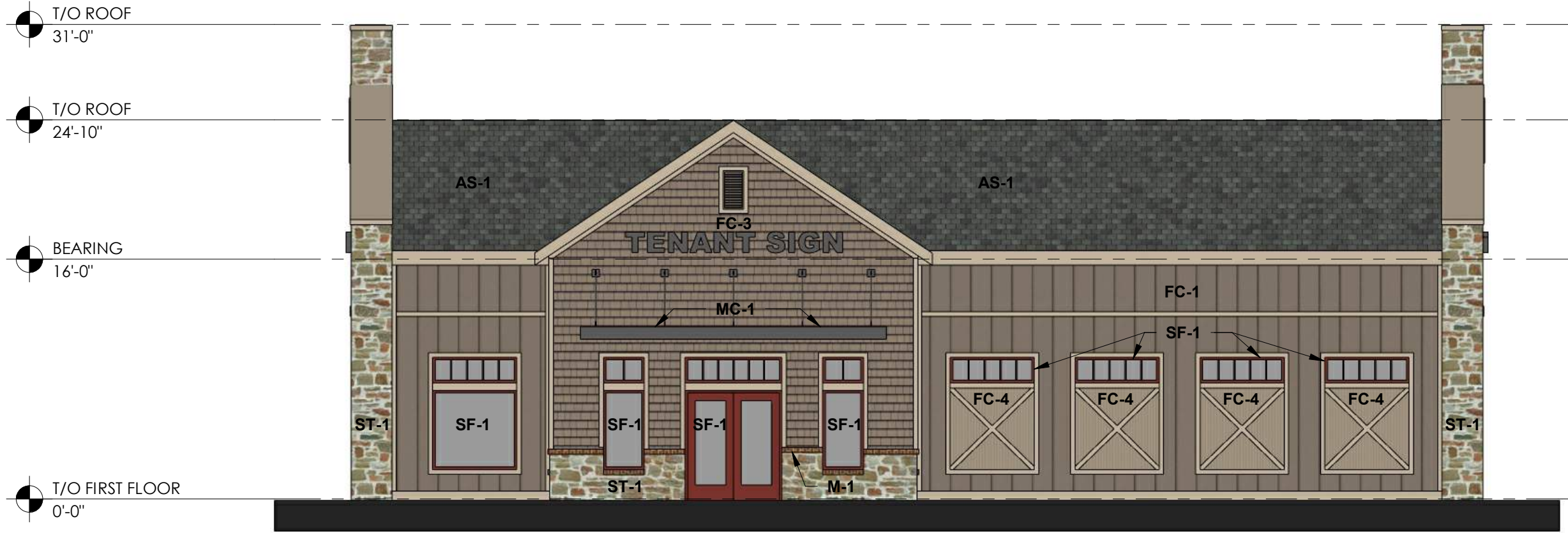
1 BUILDING C SOUTH ELEVATION 1/8" = 1'-0"
