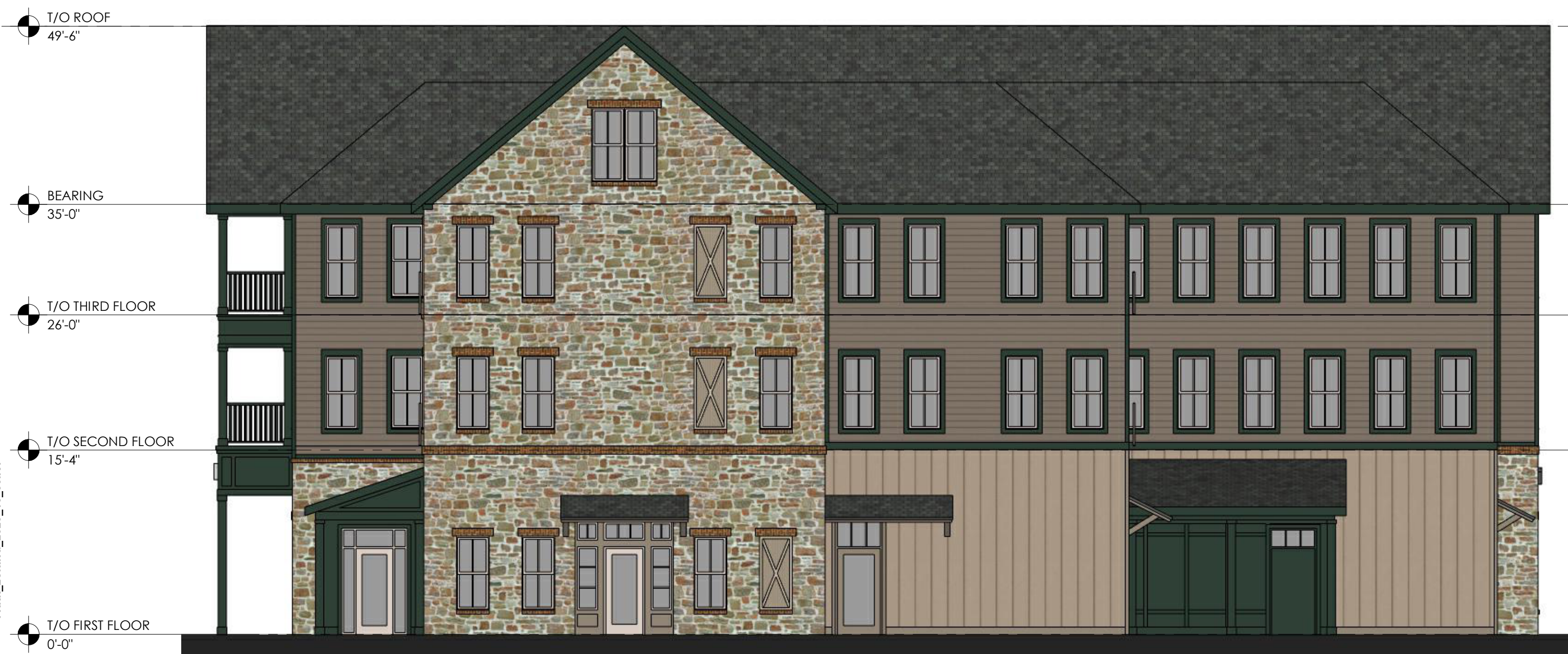
② BUILDING B NORTH ELEVATION 1/8" = 1'-0"
