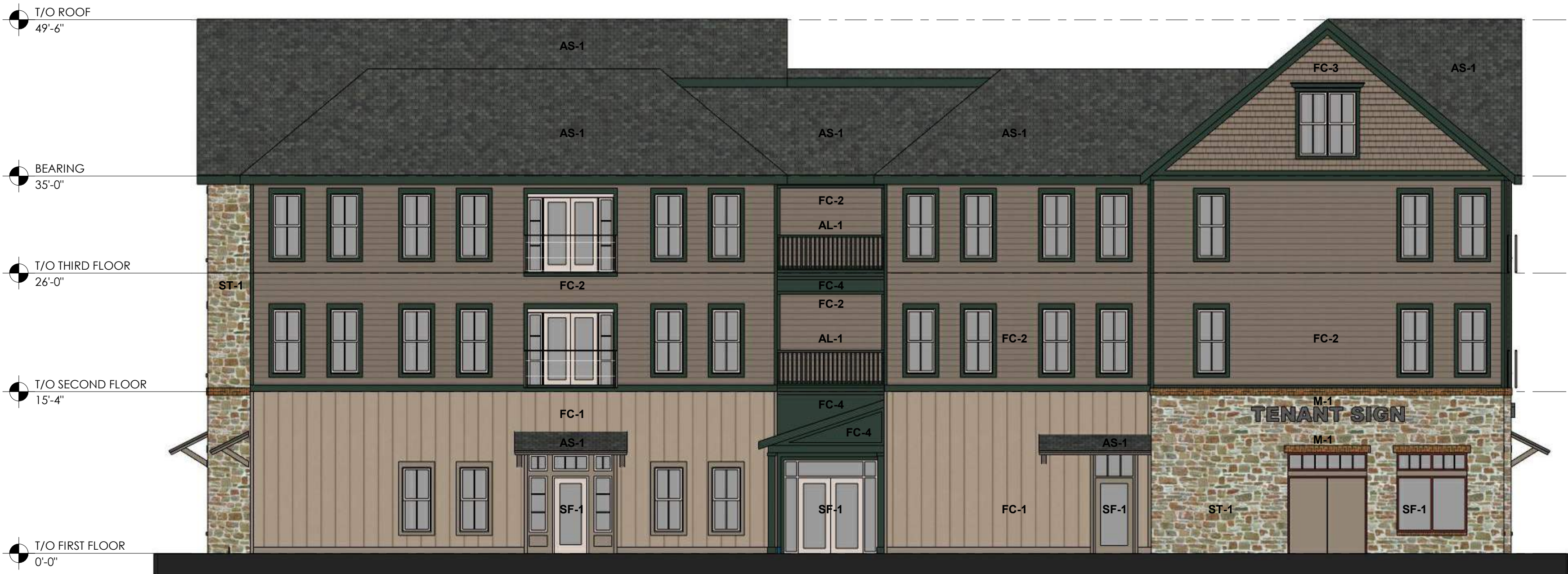
4 BUILDING B WEST ELEVATION 1/8" = 1'-0"
