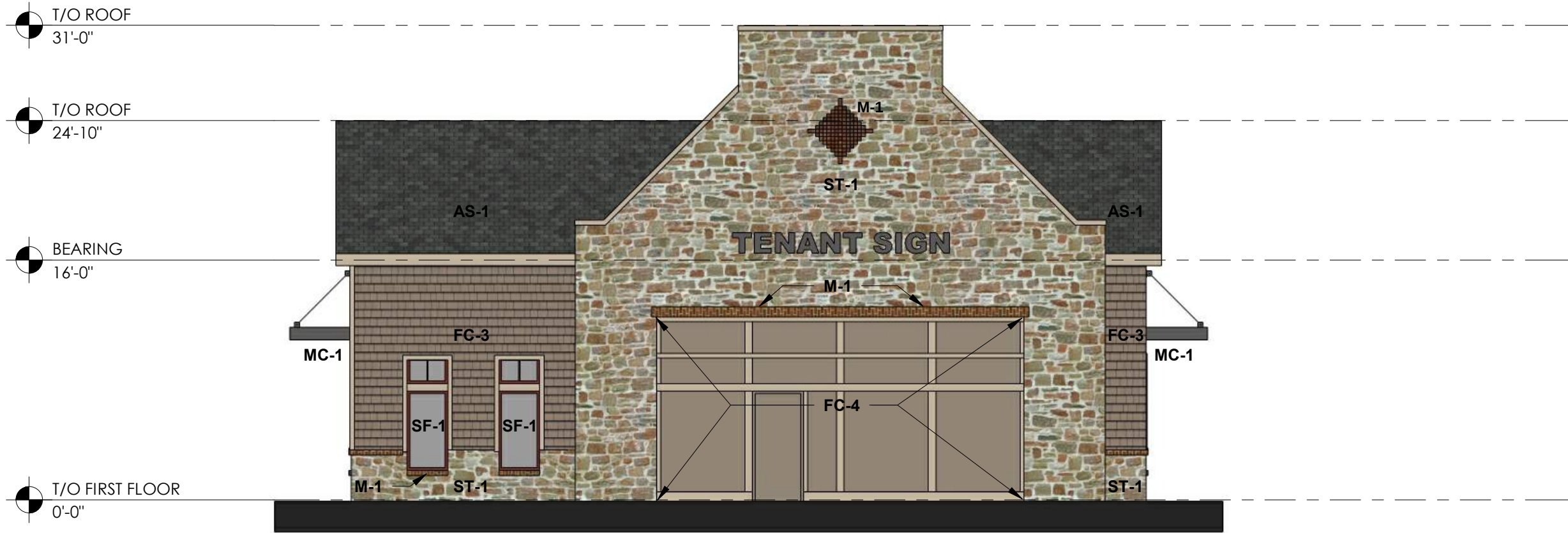
3 BUILDING C EAST ELEVATION 1/8" = 1'-0"
